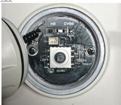
After removing the cover on the underside of the camera and with the Video Out mode switch (SW2) in the HD position, TVI is the default output. If you require AHD, then without the OSD being on, push and hold the joystick to the Left for c.5 secs, this puts the camera into AHD (the camera needs to be powered). The same process should be applied to put back into TVI mode, but by moving the joystick Right.
