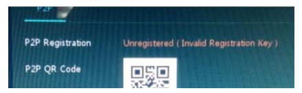
Then the device MAC address is not contained in the Server database and will need to be added.
