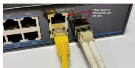
SFP installed – note copper OR fibre, not both!
