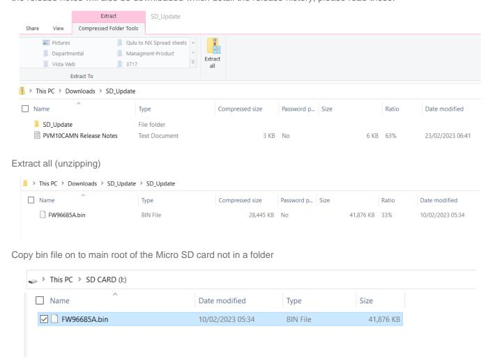
Down power PVM monitor Insert Micro SD card into Micro SD card slot on the PVM monitor and repower, the PVM monitor will upgrade then reboot.
